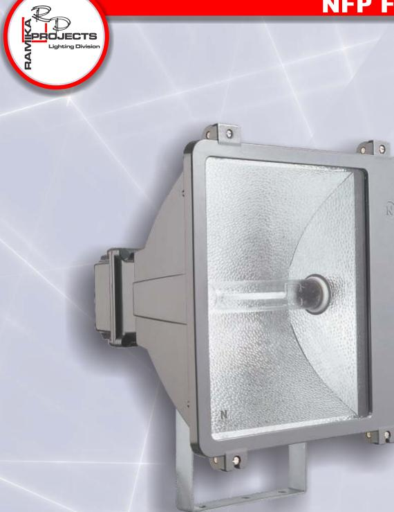
The **NFP Floodlight** luminaire range is a high-performance industrial DMC, glass fibre reinforced polyester luminaire that has been certified for Zone 2, 21 & 22 hazardous areas, and designed to satisfy a wide range of industrial and area lighting applications. It is available in HID lamps and is suitable for wall, pole and high mast installation. The **NFP Floodlight** continues the proud heritage of RAMIKA PROJECTS quality standards.
