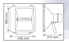
Ex-mark: Ex nA nR IIC T3 Gc IP66 Ex tb IIIC T200°C Db IP66
