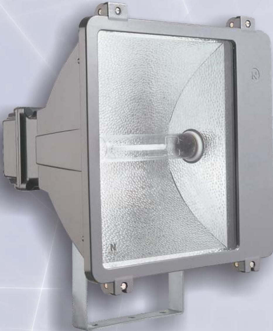
The **NFP Floodlight** luminaire range is a high-performance industrial DMC, glass fibre reinforced polyester luminaire that has been certified for Zone 2, 21 & 22 hazardous areas, and designed to satisfy a wide range of industrial and area lighting applications. It is available in HID lamps and is suitable for wall, pole and high mast installation. The **NFP Floodlight** continues the proud heritage of RAMIKA PROJECTS quality standards.
