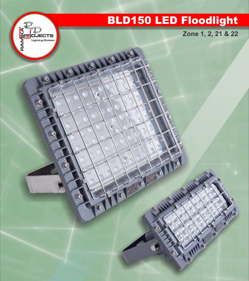
The **BLD150** is a high performance LED indoor and outdoor floodlight luminaire, designed and certified for Zone 1, 2, 21 and 22 hazardous areas. The luminaire is designed to replace the conventional HID lamp technology which makes it energy efficient with high performance, low maintenance and long life span. It's suitable for wall, ceiling and bracket mounting. The **BLD150** continues the proud heritage of RAMIKA PROJECTS Ex safety standards whilst utilizing the latest LED technology.
