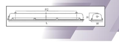
Ex-mark: Ex nA nR IIC T3 Gc IP66 Ex nA nC IIC T3 Gc IP66 Ex tb IIIC T200°C Db IP66
